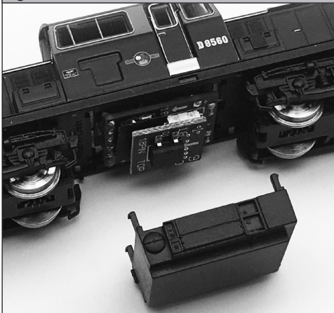
Fig.4 Push-fit Next18 DCC Decoder
