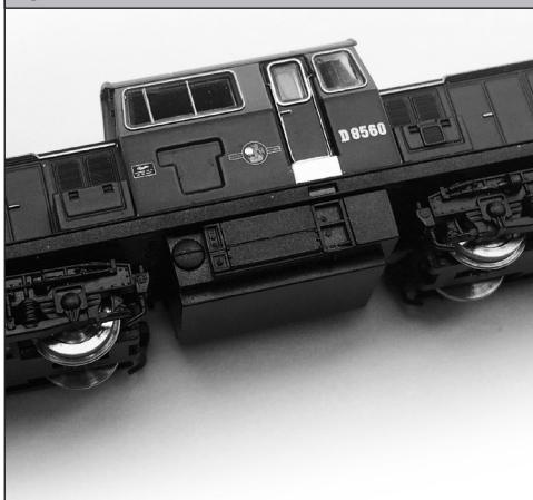
Fig.3 Remove Next18 Blanking Plate
